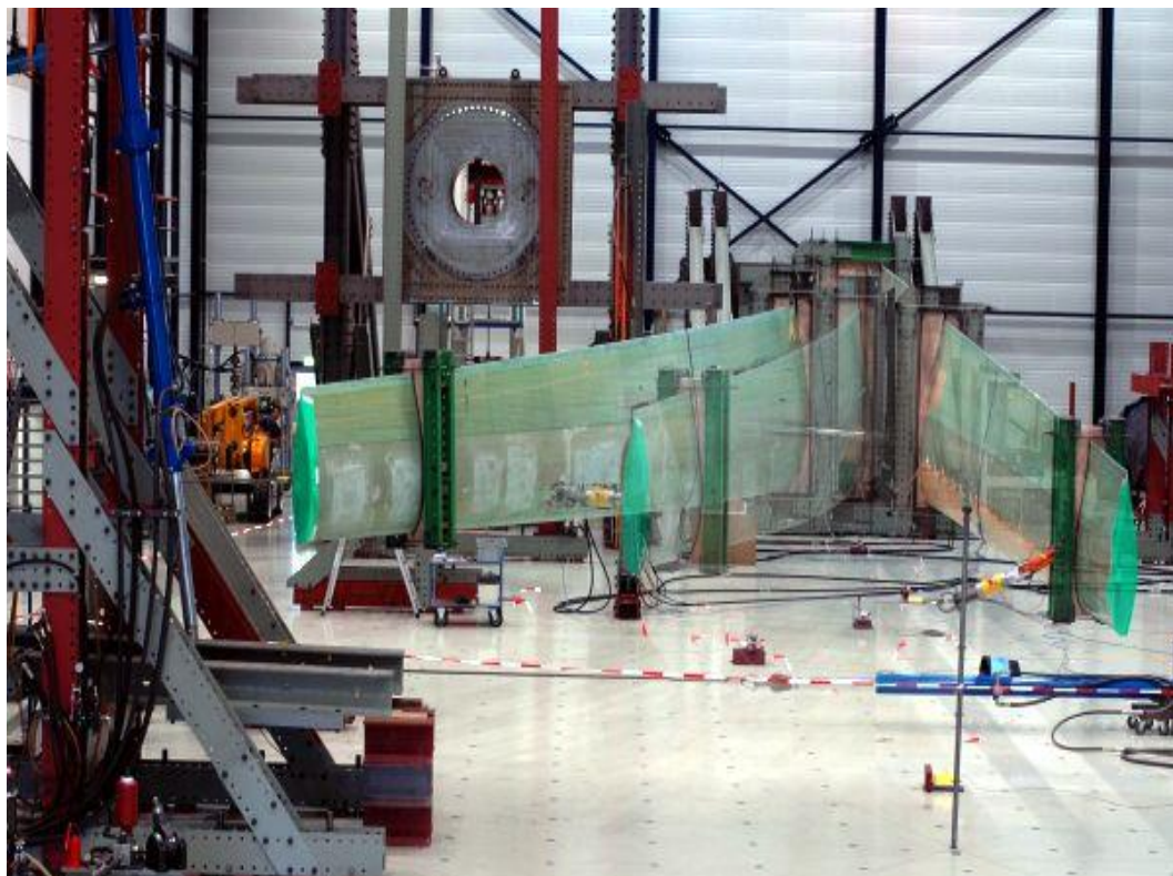
Figure 7: Triple exposure of a blade undergoing bending test.
